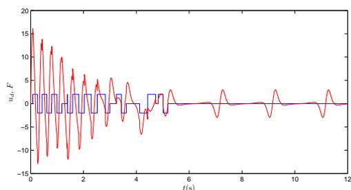
Fig. 8. Desired acceleration of the cart(blue, darker) and applied force to the cart(red, brighter).
