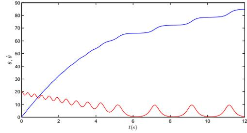
Fig. 6. Angular position(blue, darker) and velocity(red, brighter) of the pendulum.
