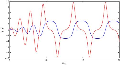
Fig. 2. Angular position(blue, darker) and velocity(red, brighter) of the pendulum.
