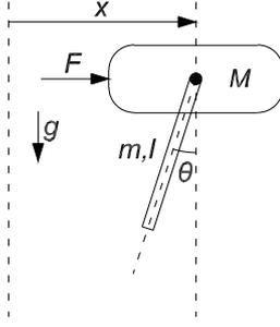
Fig. 1. Pendulum on a cart.
