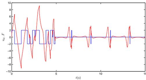
Fig. 4. Desired acceleration of the cart(blue, darker) and applied force to the cart(red, brighter).
