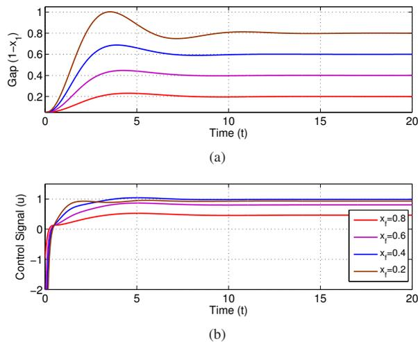
Fig. 5. Stabilization of 0.2, 0.4, 0.6, and 0.8 gap position in opening phase: (a) gap ( $1 - x_1$ ); (b) control signal  $u$ .
