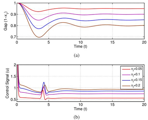
Fig. 2. Stabilization of 0.95, 0.9, 0.85, and 0.8 gap position in closing phase: (a) gap  $(1 - x_1)$ ; (b) control signal  $u$ .
