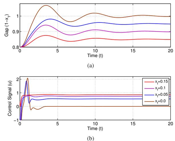
Fig. 4. Stabilization of 0.85, 0.9, 0.95, and the full gap position in opening phase: (a) gap  $(1 - x_1)$ ; (b) control signal  $u$ .
