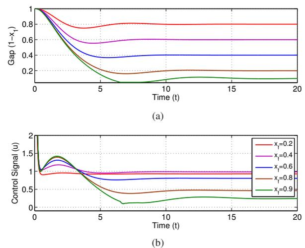
Fig. 3. Stabilization of 0.8, 0.6, 0.4, 0.2, and 0.1 gap position in closing phase: (a) gap  $(1 - x_1)$ ; (b) control signal  $u$ .
