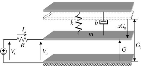
Fig. 1. 1DOF parallel-plate electrostatic actuator.
