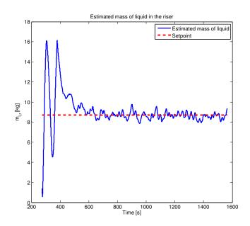
Fig. 5. Convergence of the estimated mass of liquid in the riser.
