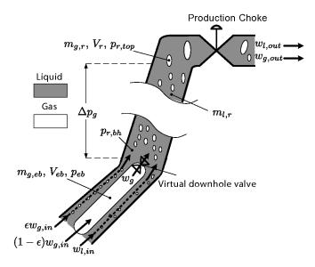
Fig. 1. Schematic representation of the transport line under consideration
