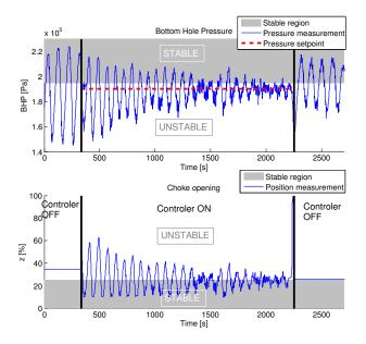
Fig. 3. Stabilization to  $RBP_{ref} = 1.9$  bar with PI controller
