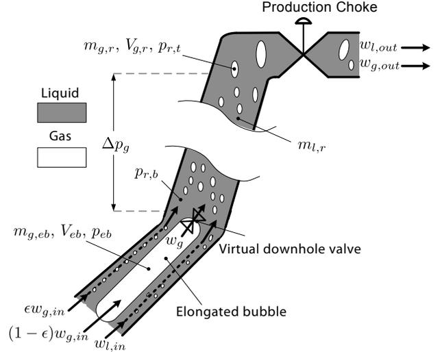
Fig. 1. Schematic view of an inclined riser carrying an inhomogeneous blend of liquid and gas
