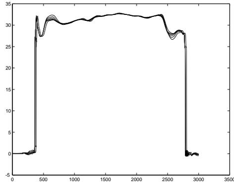
FIGURE 3. Here the signal is restored without waiting for the steady state estimate. The least squares algorithm uses the boundary matrices. The delays for the reconstructions are respectively 361, 341, 321, 301, 281 and 261. Gaining 120 sampling intervals implies a significant corruption of the restored signal
