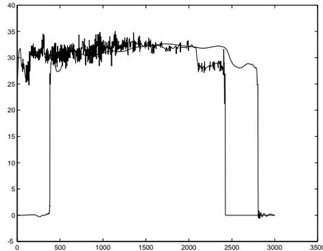
FIGURE 1. The original signal and its reconstruction with the algorithm à trous. The delay is given by  $delay = (2^{scales} - 1) * (Filterlength - 1)$ . Its value is 381 sampling intervals here.
