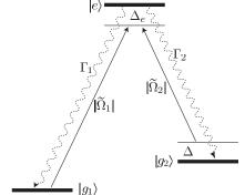
Input:  $\tilde{\Omega}_1, \tilde{\Omega}_2 \in \mathbb{C}$  and  $u = \frac{d}{dt}\Delta$ . Output: photo-detector click times corresponding to stochastic jumps from  $|e\rangle$  to  $|g_1\rangle$  or  $|g_2\rangle$ . Synchronization goal: stabilize the unknown detuning  $\Delta$  to 0. Two time-scales:  $|\tilde{\Omega}_1|, |\tilde{\Omega}_2|, |\Delta_e|, |\Delta| \ll \Gamma_1, \Gamma_2$
