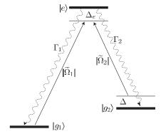
$\begin{array}{l} \textbf{Rabi frequency modulations:}\\ \tilde{\Omega}_{1}(t) = \Omega_{1} - \imath \varepsilon \Omega_{2} \cos(\omega t) \\ \tilde{\Omega}_{2}(t) = \imath \varepsilon \Omega_{1} \cos(\omega t) + \Omega_{2} \\ \text{with } \Omega_{1}, \Omega_{2} \ll \Gamma = \Gamma_{1} + \Gamma_{2}, \\ \textbf{0} < \varepsilon \ll 1 \text{ and} \\ \frac{\Omega_{1}^{2} + \Omega_{2}^{2}}{\Gamma_{1} + \Gamma_{2}} = \gamma \ll \omega \ll \Gamma \end{array}$
