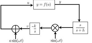
Here  $u = \omega_{diode}$ and  $y = f(\omega_{diode})$ where *f* admits a sharp maximum at the unknown value  $\bar{u} = \omega_{atom}$ .
