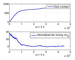
A-system parameters:  $\Gamma_1 = \Gamma_2 = 10$ ,  $\Delta_e = 2.0$ Modulation parameters:  $\Omega_1 = \Omega_2 = 1.0$ ,  $\omega = 2.8$ ,  $\varepsilon = 0.14$ Feedback gain K = 0.0023 leading to a standard deviation  $\sigma_K = 0.0057$
