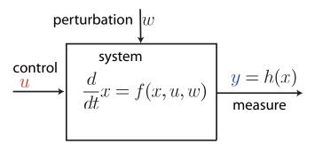
For the harmonic oscillator of pulsation  $\omega$  with measured position *y*, controlled by the force *u* and subject to an additional unknown force *w*.
