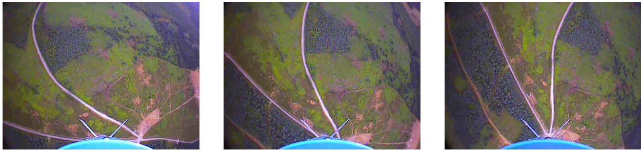
Figure 8. Potential use of the onboard camera as a rotation sensor.
