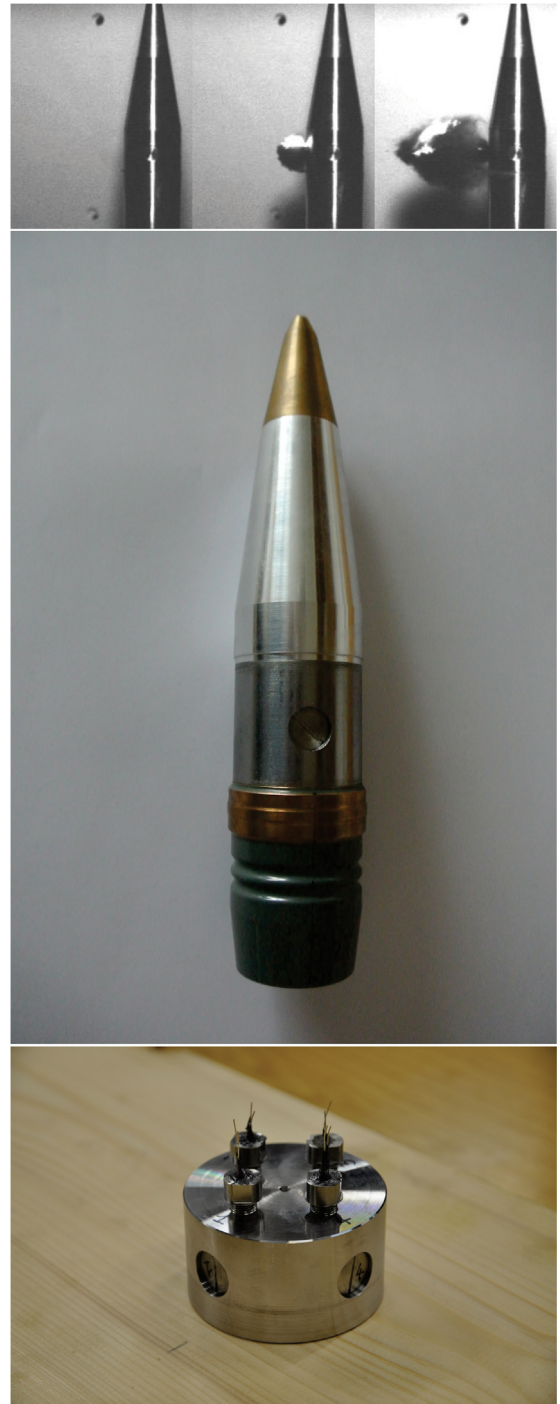
Fig. 3. ISL pyrotechnical thruster. Top: close-up view during thrust. Middle: integration in a 155 mm shell. Bottom: the thruster.
