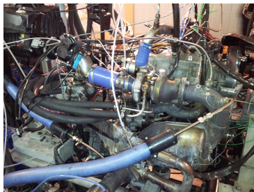
FIG.: IFPEn test-bench, 1.8L RSA F5Rt
